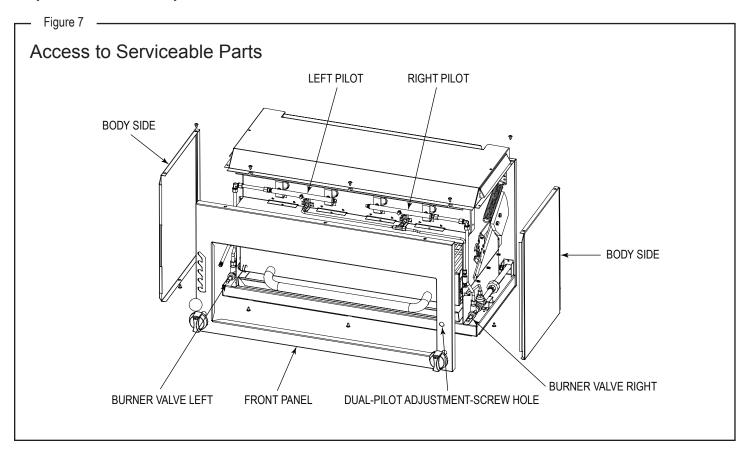
If necessary (or convenient), wall-mounted and flue-riser-mounted models can be un-mounted for servicing or repairs. Use two people since the broiler weighs about 175 pounds (77 kilograms). Refer to the installation procedure in the previous section of this manual for guidance.
